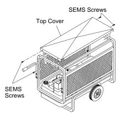
Figure 9 – Attaching Top Cover to Roll Cage
